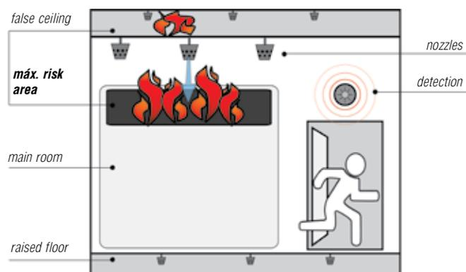
INERT-SIEX™ 100 acts throughout the volume, including all areas of difficult access, which it reaches easily without residue or particles.
